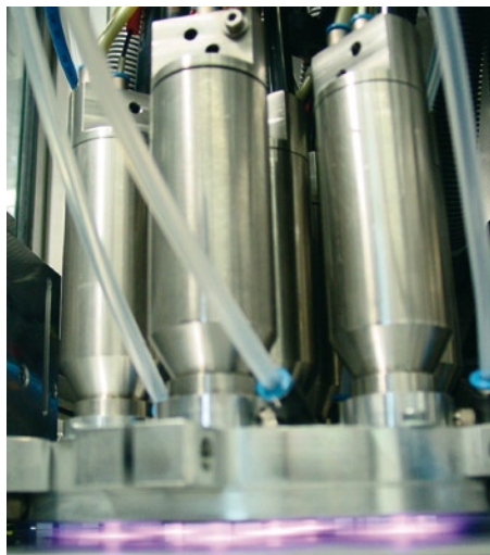
Plasma nozzle assembly for coating large-area substrates.
